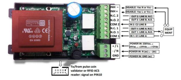
*J3 socket:* connect the coin mechanism (or the ACS RFID Card/Key reader) to the Servo-relay p.c. board using a 10-pole flat cable.
