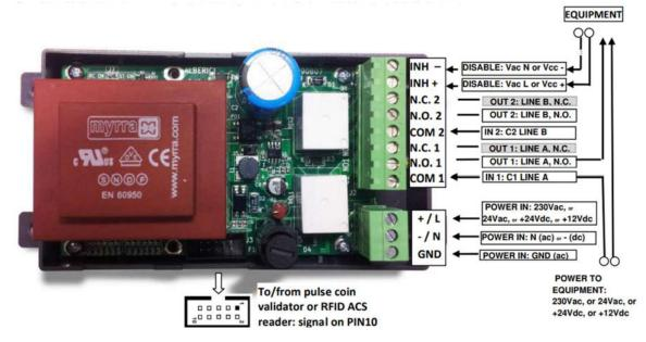
*J3 socket:* connect the coin mechanism (or the ACS RFID Card/Key reader) to the Servo-relay p.c. board using a 10-pole flat cable.
